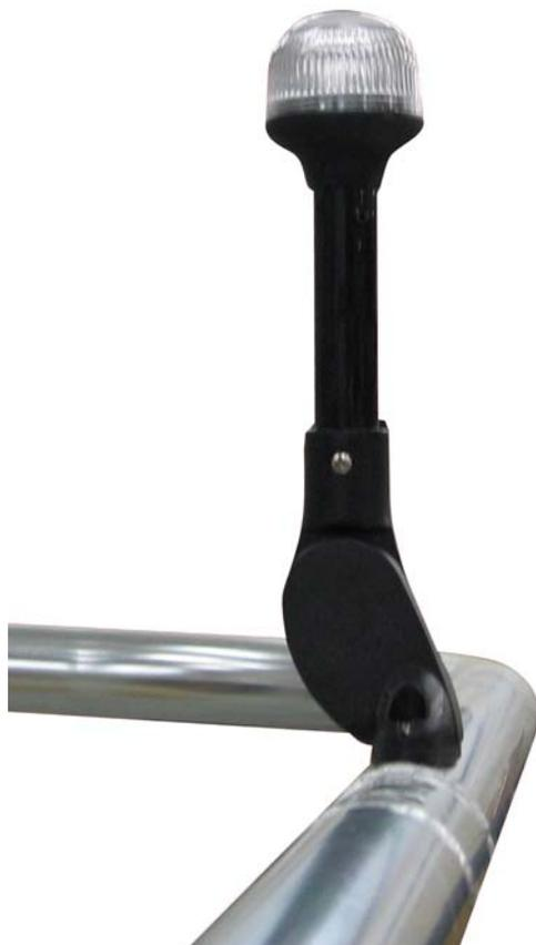
Place your light on the T-Top where you would like it located. In the above photo, it is slight off center on the back of the top. Once it is located where you want, mark the hole locations for drilling. (See following page for wiring instructions)
