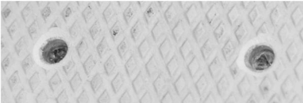
**Put 3M 5200 Adhesive in Holes and Base Location:** The 3M 5200 Marine Adhesive is a key structural part of any T-Top installation. Squirt 5200 into each hole and be sure it is filled with 5200. Then add a smooth layer about 1/16" thick between the four holes. The majority of the strength comes from the screws being bonded to the hole and the base being bonded to the deck adds additional strength. This should look like the image below.
