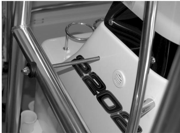
**Use the 3/8" bit to drill through the T-Top leg and center console as shown. Use a center punch to locate the hole on the tube and drill first with the 11/64" bit. If needed you can drill the hole in the console from above and below the cross tube. If you do this first drill from both directions with the 11/64" bit then both directions with the 3/8" bit.**
