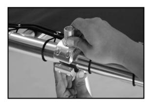
3. Insert socket Head Cap Screws and tighten.
