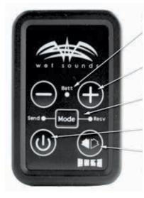
**Battery Indicator** - Solid Red when charging, when the LED is out the unit is fully charged
