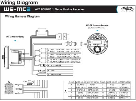
Wet Sounds WS-MC2 1 Piece Marine Receiver Operations / Installation Manual
