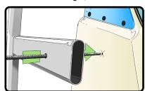
Measure standoff and cut with 4. a fine tooth handsaw to the appropriate length.
