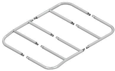
2. Install bolts to join the canopy sections together.
