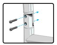
3. Insert the metal washer followed by the hinge bolt into the hinge.
