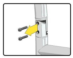
Screw in one Quick Release Knob in top 2. or bottom hole on leg section. There will be an open hole on each leg.
