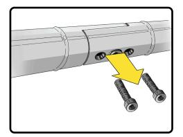
2. Replace bolts with 2 Quick Release Knobs. Repeat on other side of tower.
