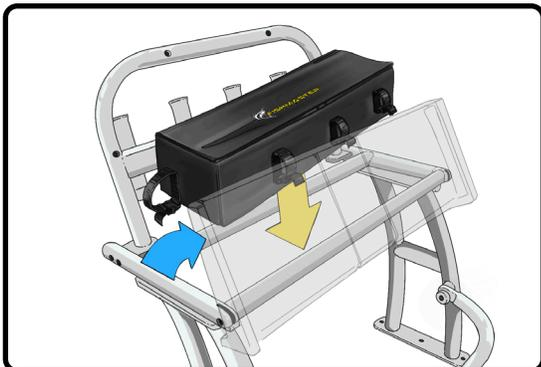
2. Attach each buckle strap to the frame of the leaning post.
