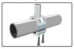
2. Slide the mounting plate onto the post, apply thread locker, then tighten down the bolts.
