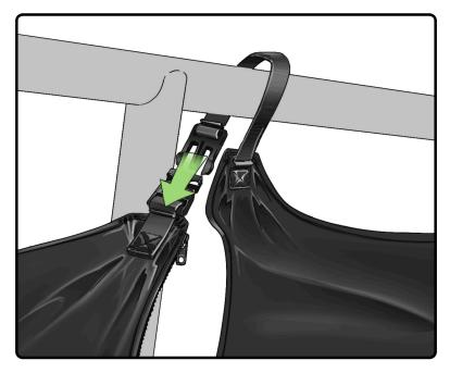
Locate the strap, place over the t-top frame, and clip it to the buckle.
