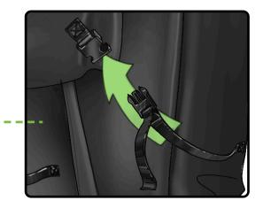
Connect the side straps to the buckles located on the front of the center flap.
