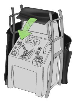
Locate the center flap and place it over the center console.
