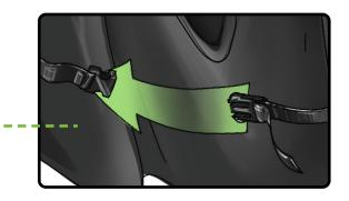
Connect both the top and bottom center buckles together. These will pull the fabric closer to the console.
